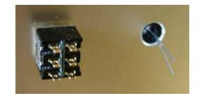
(above) The front exists of two separate panels. The switch will be mounted on the inside panel. In the thick front plate we drill a hole that is big enough to move the axel freely. I used a long toggle switch (bought from Conrad). The LED holder is mounted on the front. Drill a somewhat bigger hole in the back panel to prevent a short circuit.
