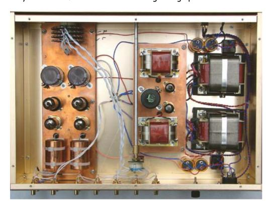
Next to that: a closed enclosure can also be nice and handy to use, surely when we are talking about a line amplifier. For power amplifiers I like the old fashion 'on top' setup by far and in addition to that; it is the most practical way to go with the large transformers and tubes on top of the chassis and the wiring and components below..
