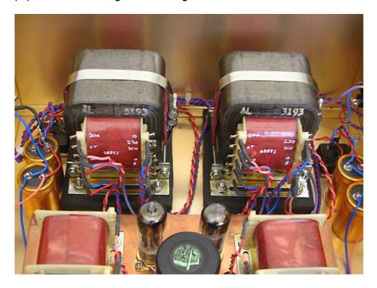
There will be used a pair of special luxury band core power transformers and the same quality amorphous core chokes as applied in all the other amplifiers. The power supply has to "stand up" right away and will be built from the specs obtained from Duncan PSU designer. The Classic One line amplifier has a relative low voltage of 225 volts (DC)..
