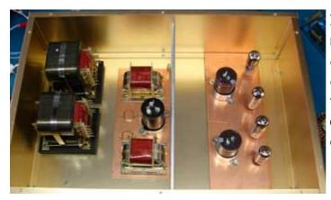
It always starts out with measuring and fitting. Here you can see the 3 separate components, The power transformers, the power supply and the amplifier. Each on its own sub chassis.
