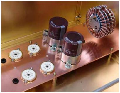
The parts can be mounted now. The elco's will be mounted with the well known clamps.
