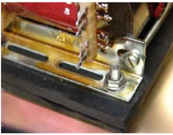
A detailed view of the mounting brackets of the power supply transformer. I glued 2 thick rubber flaps together. Before gluing them together, one half is used to glue-in the bolts for mounting it to the chassis. The other half is used to glue in the bolts for mounting the transformers. With this, the transformers are nicely mechanically decoupled from the chassis. As it later turned out,
