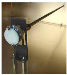
To avoid a thick bundle of sensitive input cabling from the back to the front, the input selection switch is placed as close as possible to the RCA input connectors. The switch is operated with a long axel. That's a task of precise outlining to prevent mechanical stress. The long holes in the mounting profile are helping out.
