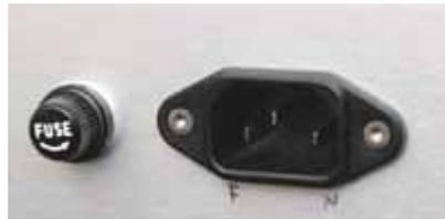
The inlet for the power cable and of course the necessary circuit breaker.
