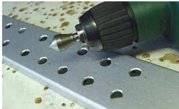
The holes for the cinch busses. Pre-drill with 3 mm, than drill up to 9,5 mm. Clean the edges for a nice result.
