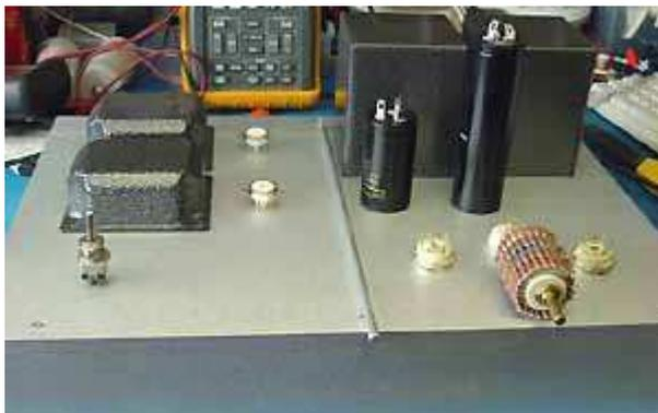
The parts are placed with a lot of fitting, measuring and moving their definite position on the chassis. I keep the same lay-out as I previous used on the Cleo-V, what results in a logical wiring method for this amplifier....
