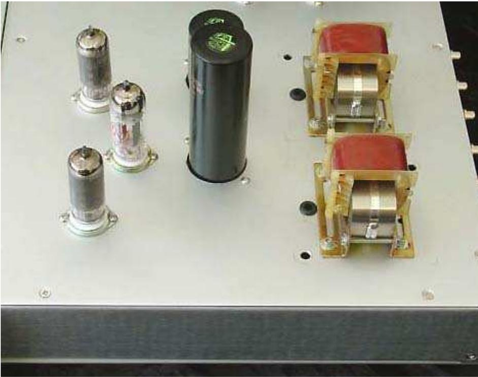
Two of the four chokes (the 15 Henry) are mounted on top of the chassis. The two inside the cabinet are the 10 Henry chokes which are placed direct behind the first PSU capacitor. On the picture below here, you can see the Icar MKP capacitors which are glued tot the chassis with some silicon kit.
