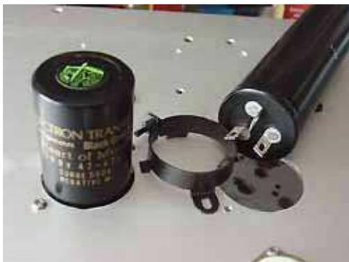
... don't leave much room for questions, is my personal opinion. Direct after the rectifier we use a 10 uF MKP in oil capacitor, an amorphous choke, a 47 uF *Black Gate WKZ*, the second amorphous choke and a 100 uF *BeeGee WKZ*. You can't find better PSU for this amplifier, exclamation mark. Yes but... eh...what about the *non-polar Black Gate NX*? That's also a nice one? Yes it is! But not for the high
