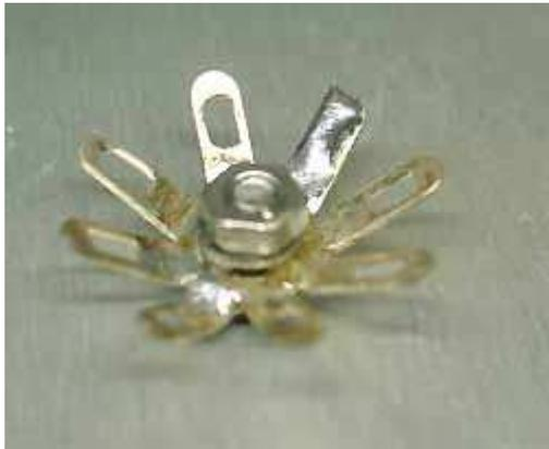
The central mass terminal is made by using several solder connectors and a small bolt. Mount it very tight, a clean good contact is a must. I always use wrinkled washers, which are digged in the aluminum.
