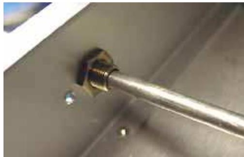
The holes for the volume pot- and input selection switch axles getting their axle sockets....
