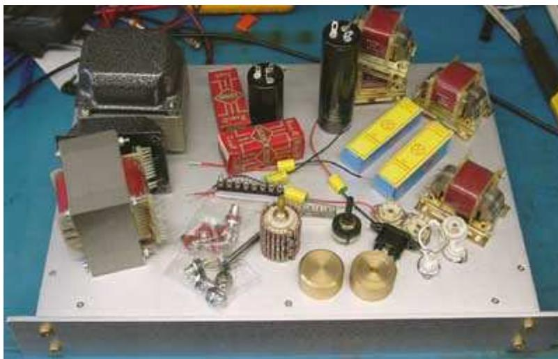
relative easy pre amplifier to build. I will use a complete aluminum chassis this time, in which I only have to drill the holes in. That may seem a big job, but the aluminum is an easy to handle metal. Because of its high quality, the drilling and punching leaves us with nice and clean holes. To drill holes with a manual
