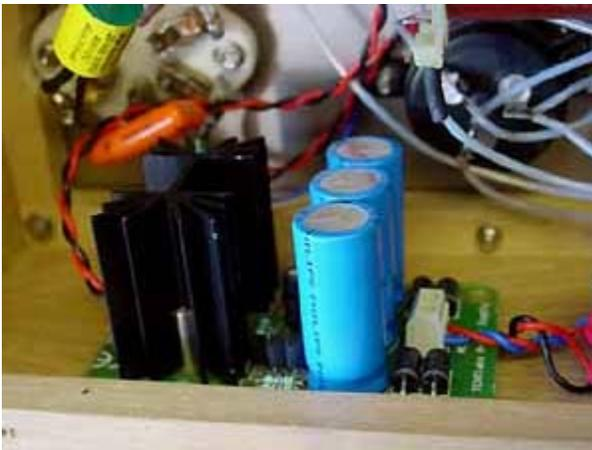
The module remains floating, its' output goes directly to the tube socket. It is up to you whether you connect the "+" or "-" side to ground (or cathode resistor in case of auto-bias). It is not yet very clear what is preferred, but ofcourse you can try it yourself and fix it afterwards.
