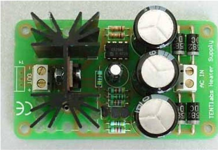
There is many ways to supply the required power to directly heated tubes, especially when discussing output tubes. When discussing pre amplifier tubes, mostly DC voltage is the only acceptable otherwise hum becomes a likely problem.
